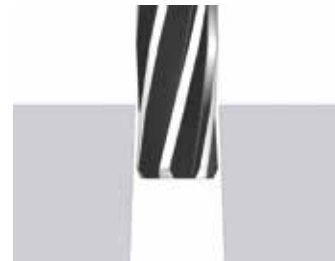
Conical bore (end too large)
