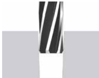
Conical bore (entry too large)
