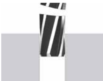
Reamer jams and breaks
