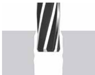
Poor surface quality
