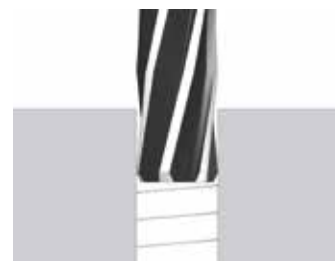
Hole shows chatter or retention marks
